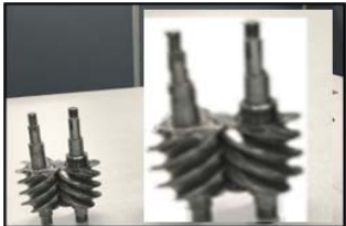
Relative Size of Compressor Screws in High-Capacity Thermal Unit Vs. Prior Unit
